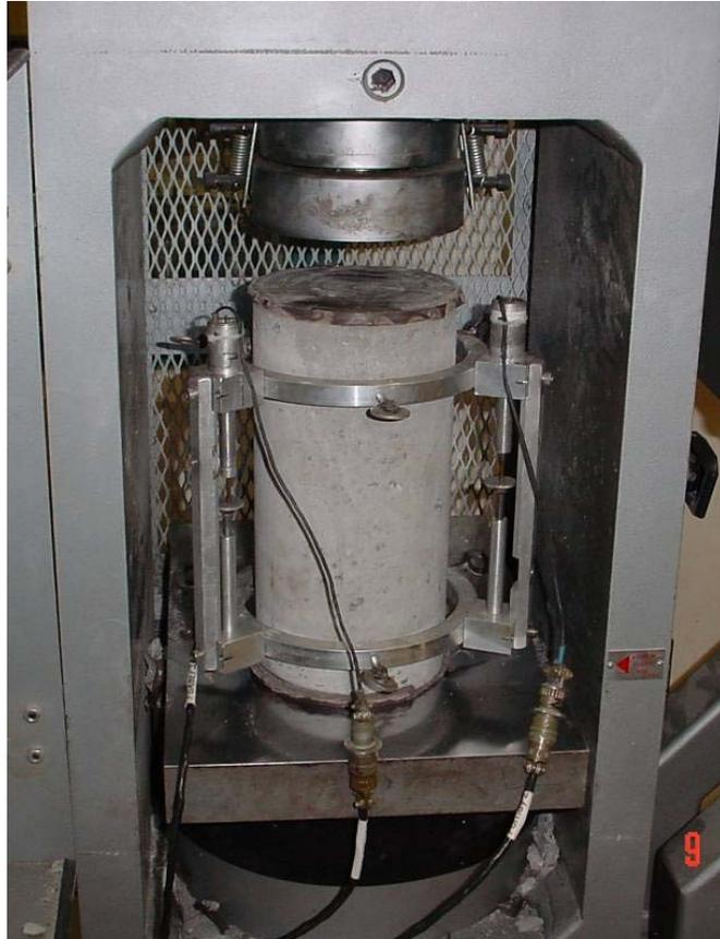
**Figure 3.16 – Compression test setup for capped 6” diameter cylinders using 3 LVDT’s and a Forney Compression Machine.**
