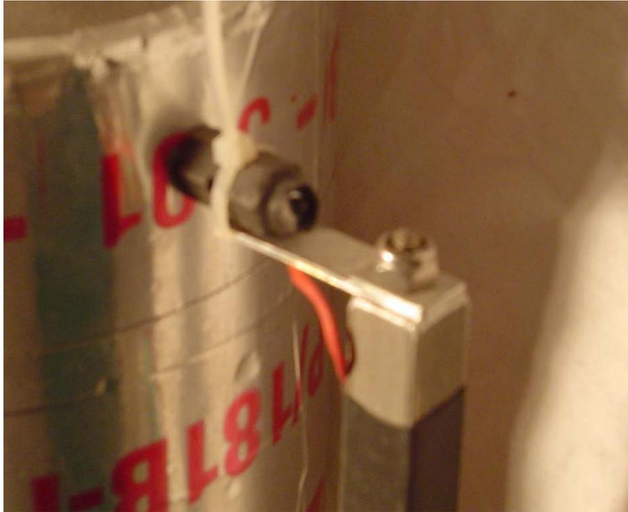
**Figure 3.20 – Close-up view of extensometer attachment to stud screwed into brass insert cast in concrete cylinder (Earney 2006).**
