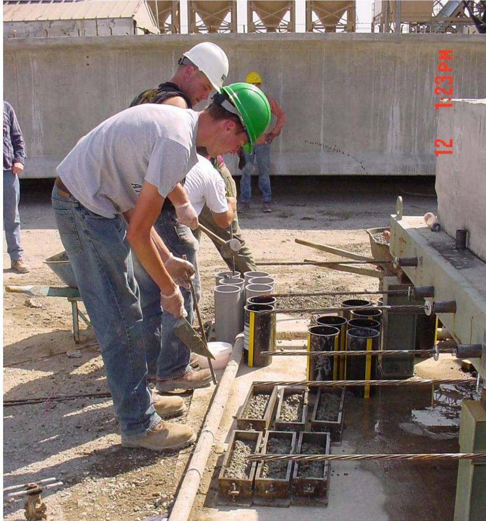
**Figure 3.18 – Creep and shrinkage cylinder casting during instrumentation trips to the precast yard.**
