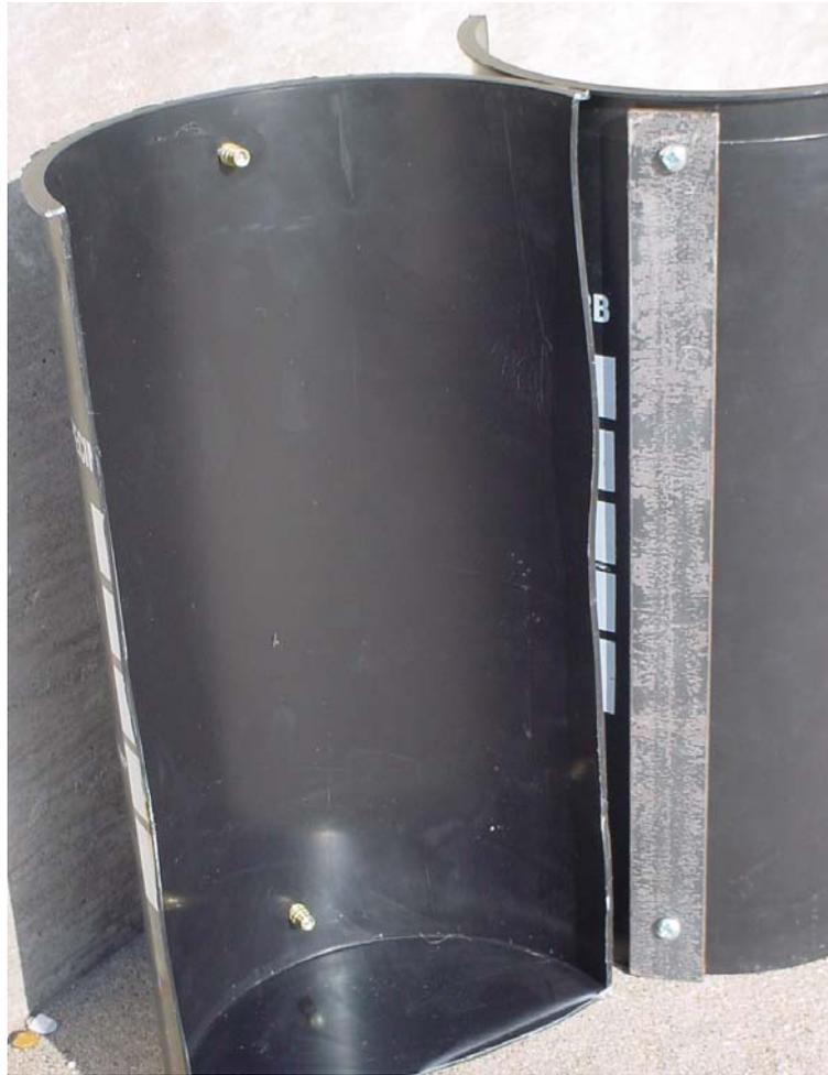
**Figure 3.17 – Interior and exterior view of cylinder molds used for creep and shrinkage. Brass anchors and spacer bars are seen (Earney 2006).**
