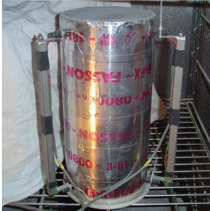
**Figure 3.22 – Sealed shrinkage specimen with three extensometers attached for measurement of shrinkage strains (Earney 2006).**
