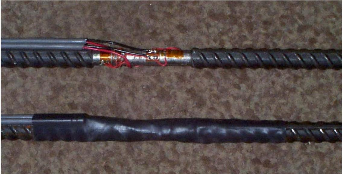
**Figure 3.5 – A completed strain-gage bar along with an instrumented bar yet to be waterproofed and sealed (Eatherton 1999)**
