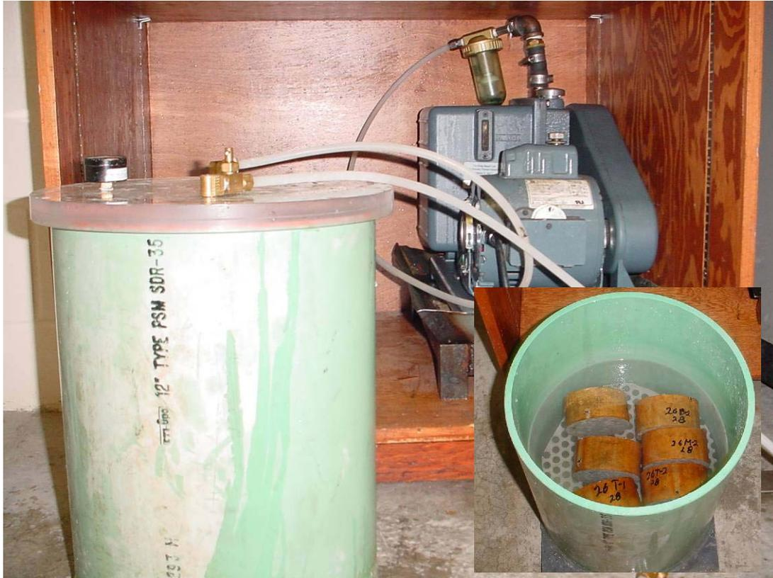
**Figure 3.26 – Photograph of the rapid chloride penetration test specimen conditioning equipment**
