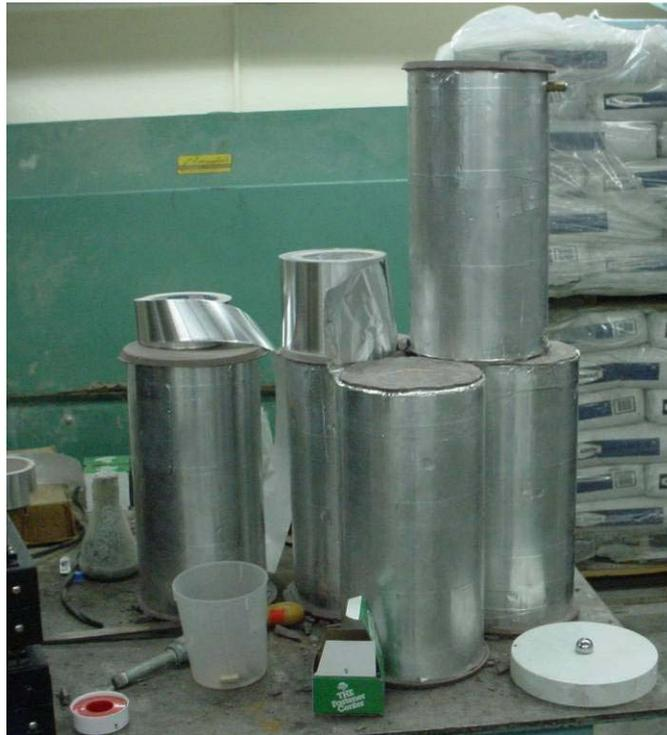
**Figure 3.19 – Picture of capped and sealed specimens used for creep and shrinkage studies (Earney 2006).**
