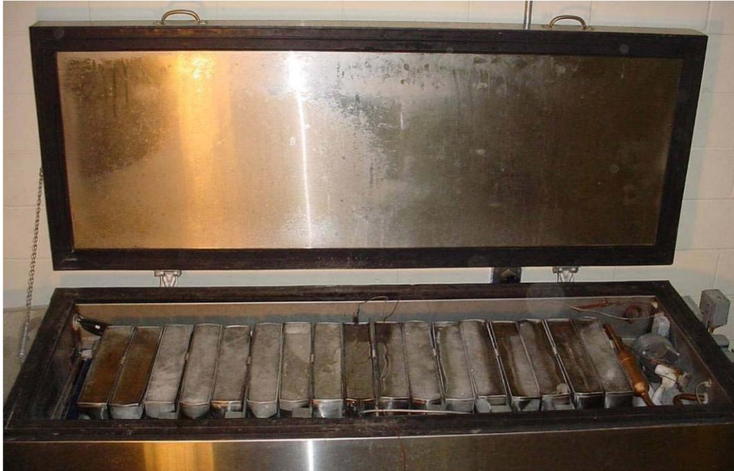
**Figure 3.27 – Overhead view of cabinet used to subject prisms to freeze-thaw cycles.**
