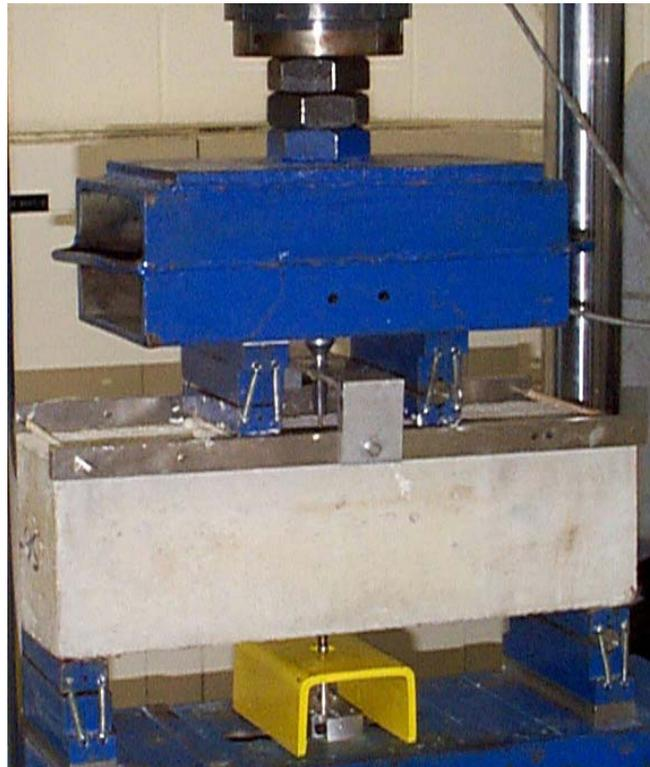
**Figure 3.29 – Photograph of third point loading of concrete prism/beam.**
