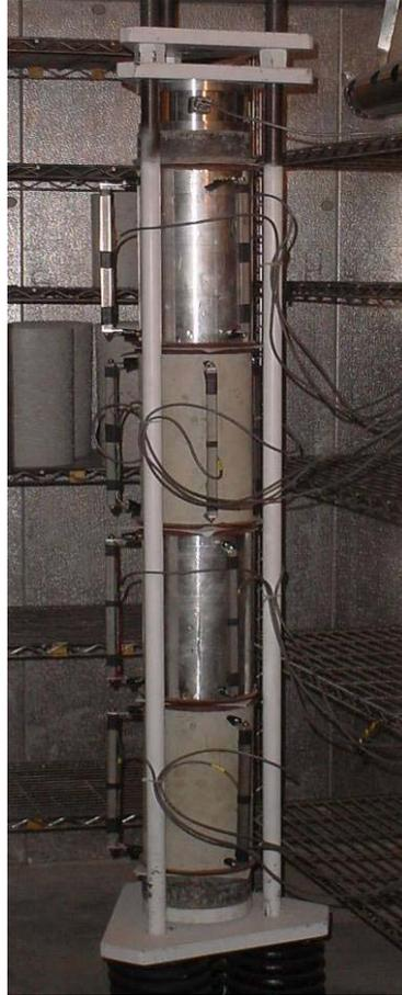
**Figure 3.21 – Creep load frame with two sealed and unsealed specimens loaded in compression (Earney 2006).**
