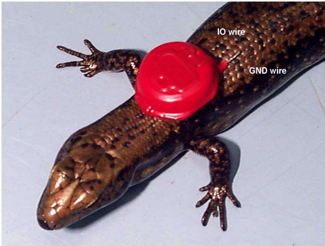
Figure 3.1. Modified data loggers were attached to the dorsal surface of female Eulamprus tympanum , between the shoulder blades. The exposed wires (IO & GND) allowed data retrieval while the logger remained attached to the lizard (see Appendix 1 for details).
