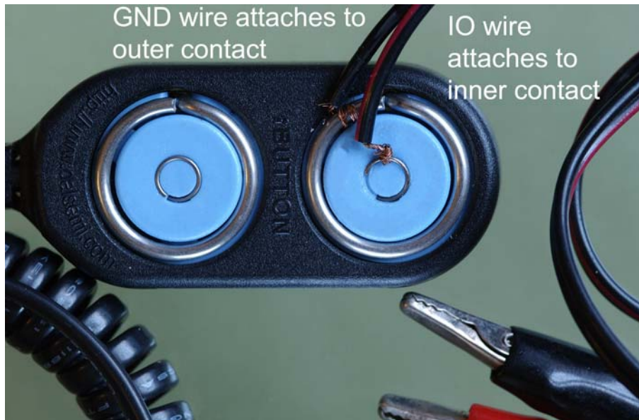
Figure A1.3 Reader (Blue Dot Receptor ® ) with wires that attach to exposed leads on the modified units via alligator clips.
