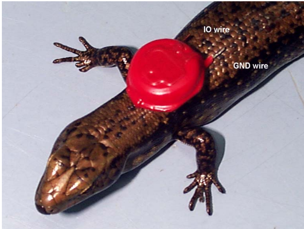
Figure A1.4 A female Eulamprus tympanum fitted with a modified Thermochron iButton.
