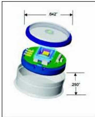
Figure 1. Illustration of the HygroChron data logger shows the small size of the canister and how an outer filter allows water vapor to reach the device's internal humidity sensor.
