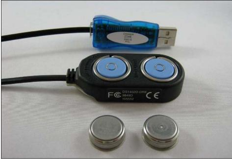
Figure 1. From front to back: logger iButtons, a Blue Dot™ receptor, a USB adapter.
